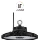
TITAN HIGHBAY MULTIFLUX 100-120-150-200W 16000-30000 LM 4000K RA80 160LM-W 120° IP65 IK08 CLI NDIM NOIR 50000H 5ANS L80B10 220-240V 50-60Hz CORPS ALU PRE CABLAGE 1,2M
